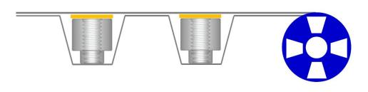
The Kapton® tape is attached to the top hole of the SMD fastener for SMT nozzle pick & place process
